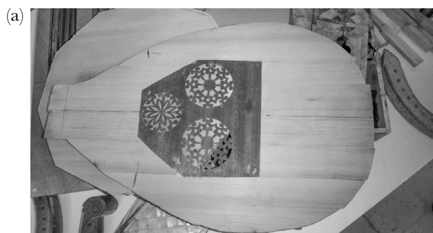
FIGURE 5a. The soundboard with the wooden reinforcement. Photo by the author.
