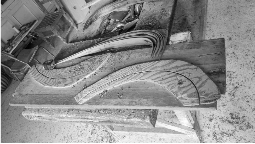
FIGURE 8. Table to shape ribs for the mold in Ridha Jandoubi's atelier. Photo by the author.
