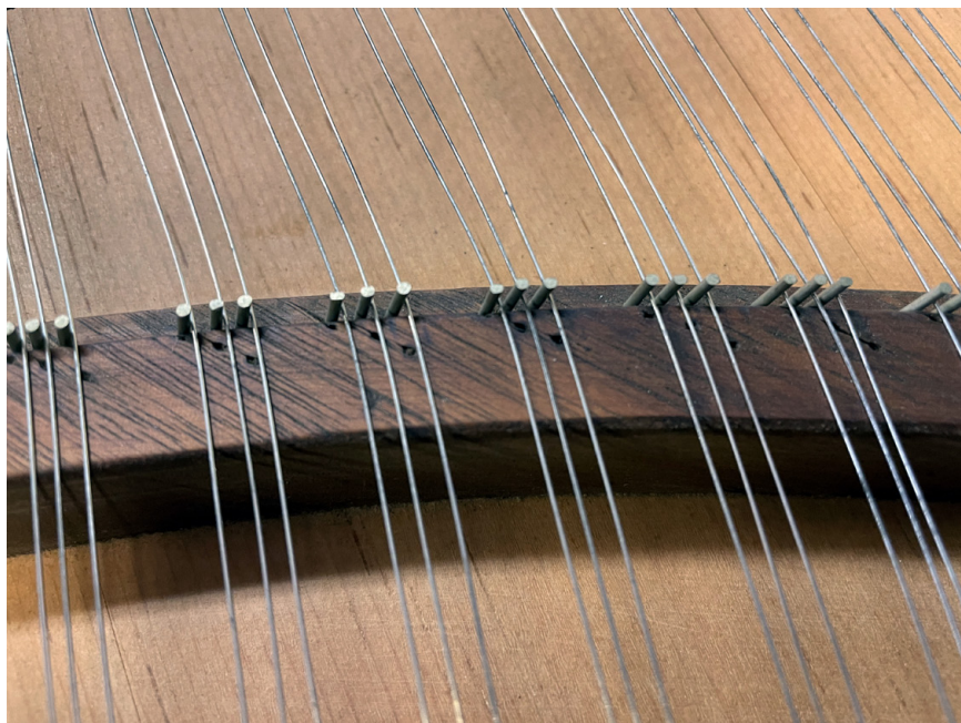
FIGURE 18. Treble bridge section of the Berent piano, showing witness holes for former back-pins.
