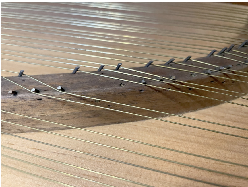
FIGURE 20. Bass end of the Berent piano bridge, showing moved back-pin witness hole, and witness holes for a double back-pinning.
