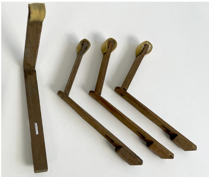
FIGURE 27. Hammers and shanks of the Berent piano's second action.
