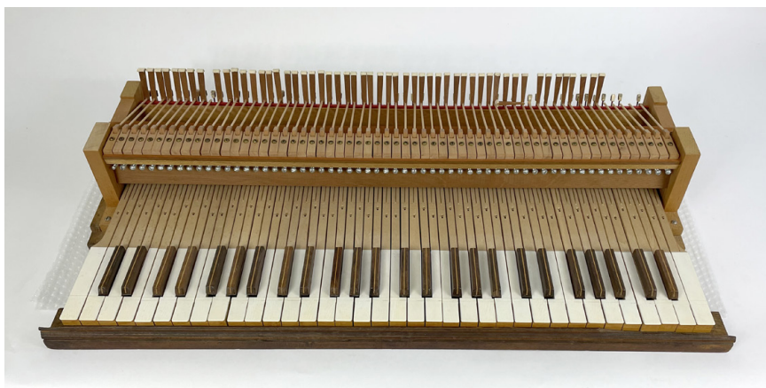
FIGURE 28. English grand action, made by Philip Belt for the Berent piano.
