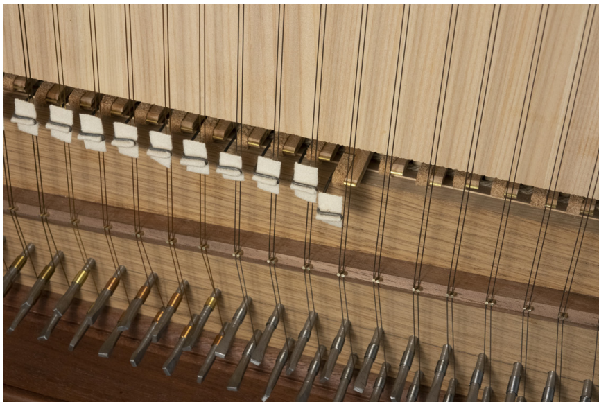
FIGURE 7. Detail of hammers and dampers in the reproduction. The top damped note (f#) is shown striking the strings, as the brass-tipped side of the hammer makes contact. The dampers are held by stiff wires attached directly to the hammers. Photograph by John R. Watson.
