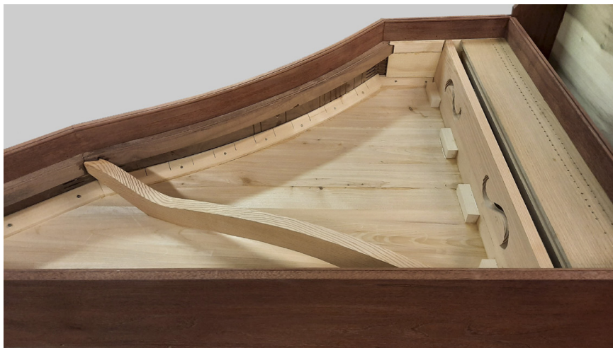
FIGURE 4. The reproduction case showing the soundbox interior before addition of the soundboard. Note the single serpentine strut, heavy liners on the bentside, and normally hidden S-shaped holes cut into the belly rail, all features based on the original instrument interior as observed through a borescope. Photograph by John R. Watson.
