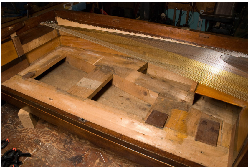
FIGURE 6. Thomas Loud piano key bed with discrete wooden pieces. Private collection; photo courtesy of John R. Watson.
