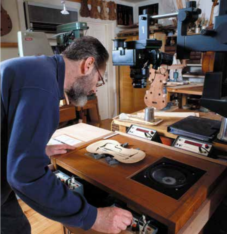
FIGURE 11. Rubio using his “shaker table” and overhead camera to capture the vibration patterns on violin plates, Cambridge, 1990s. Author’s collection.
