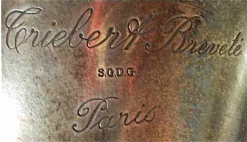
FIGURE 42. Text I, brevete B-6, and SGD.G from tenor saxophone 195. On brass-bodied woodwinds, the scripted marks are identical but at different sizes, implying pantographic engraving.
