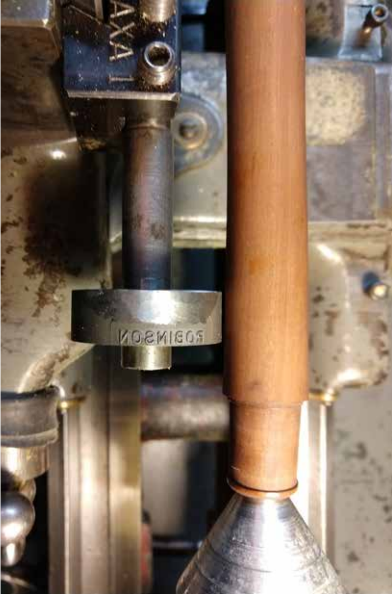
FIGURE 7. Parallel axis used with lathe to create a circumferential stamp. Courtesy of Joel Robinson.
