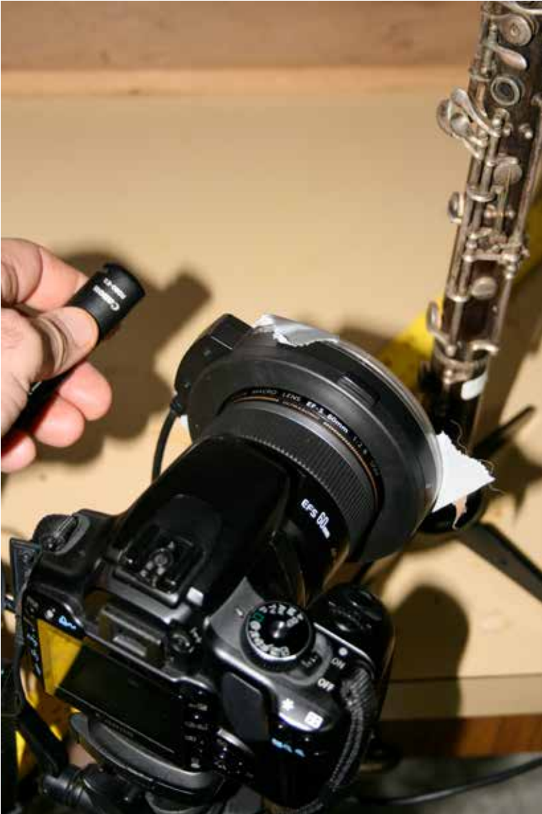
FIGURE 5. Photographic setup. The object is 9 cm from the front of the lens.
