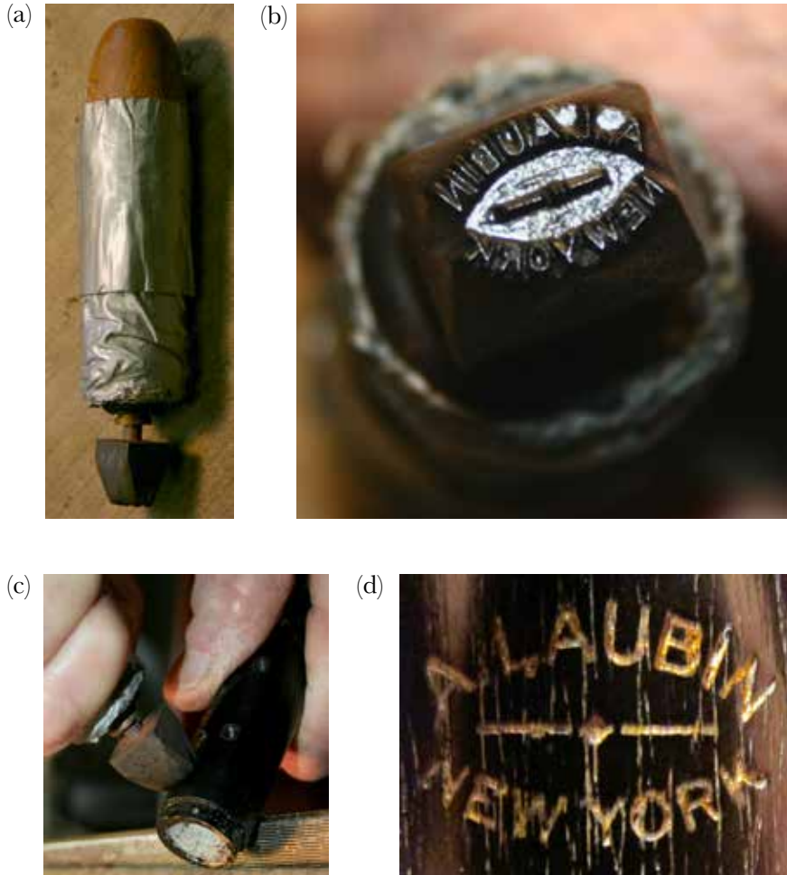
FIGURES 6a–d. Hand stamping a mark: (a) the stamping tool; (b) the working face (“die”) of the stamp; (c) applying the die; (d) the finished mark, after filling with gold wax. Courtesy of Alex and Paul Laubin.
