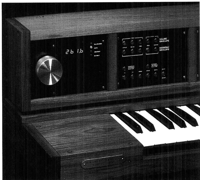
FIGURE 5. Synclavier I control knob, display window, and first button panel. Photo from a 1981 NEDCO promotional poster.
