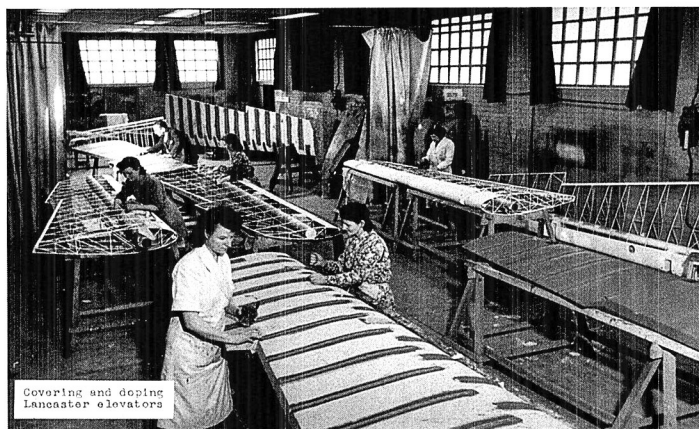
FIGURE 9. Covering and doping Lancaster elevators (HM B&H ARC/BH/BOO/012/001/001/027). Permission of the Horniman Museum, London
