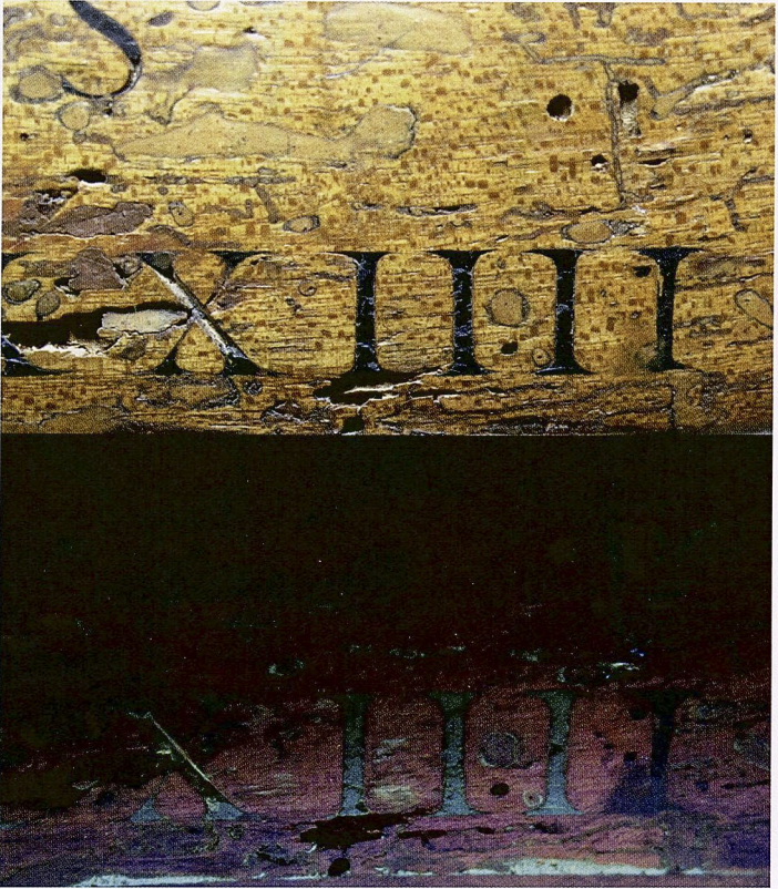
FIGURE 14. Visible light and UV image of the date, inlaid on the front panel above the keyboard. The different fluorescence of the last letter is clearly visible. Photo by Jean-Philippe Echard, © Cité de la Musique.
