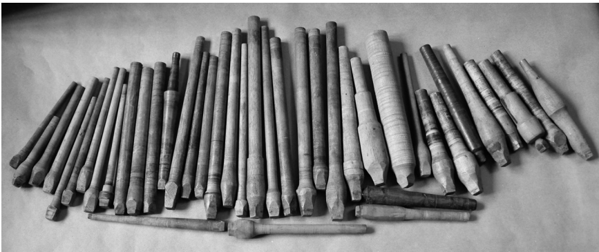
FIGURE 24. Mandrels for flute and clarinet sections of all sizes. Photo by Robert E. Eliason before the collection was moved to Oberlin in 2009.
