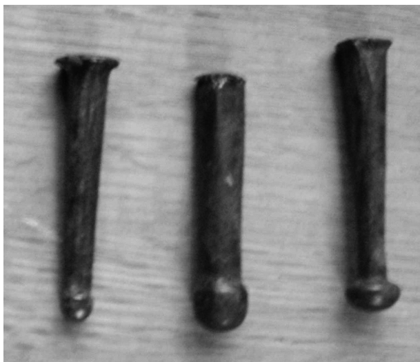
FIGURE 28. Dapping punches. Photo by Robert E. Eliason before the collection was moved to Oberlin in 2009.
