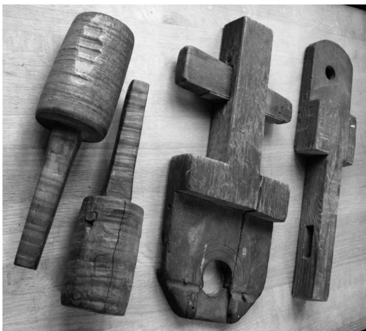
FIGURE 26. Great wheel lathe pulleys and stocks. Photo by Robert E. Eliason before the collection was moved to Oberlin in 2009.
