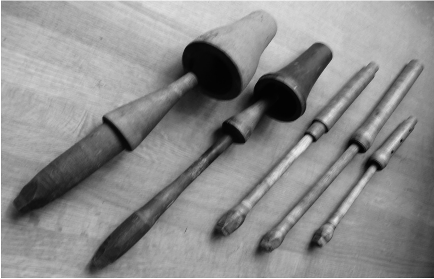
FIGURE 23. Mandrels for clarinet bells and small flute sections, with the bells and sections they fit. Photo by Robert E. Eliason before the collection was moved to Oberlin in 2009.
