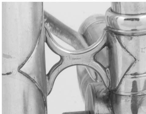
FIGURE 5. Graves & Co. Boston E-flat cornet, detail of brace and foot plates. Photo courtesy of the Montour County Historical Society, Danville, Pennsylvania.
