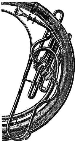
FIGURE 52b. Valve tubing of a helicon bass in BB-flat in the Illustrated Catalogue of D. C. Hall , 1876, detail of page 16.
