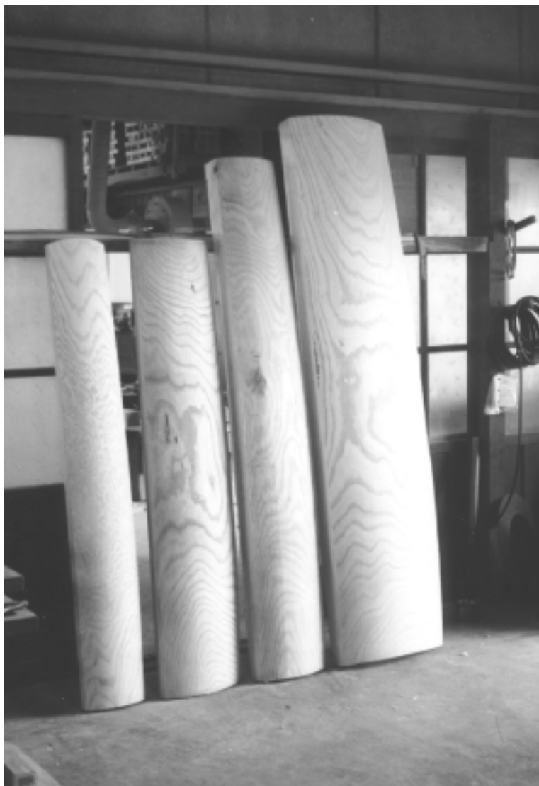
Figure 14. Instruments during manufacture at Mitsuya koto factory. Left to right: koto , nijūgen , jūshichigen , sanjūgen . Saitama, June 1998.
