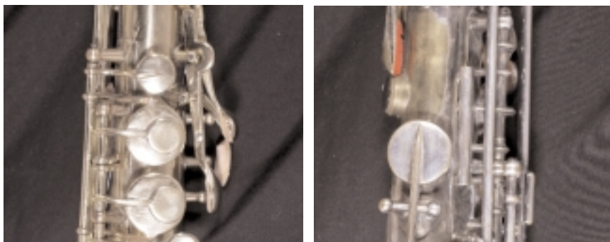
Figure 4. Left, key linkages, Adolphe Sax alto saxophone no. 21494 (1861). Right, the same key linkages on Adolphe Sax fils tenor saxophone (c. 1890), showing the modern form. Both instruments from the author's collection.
