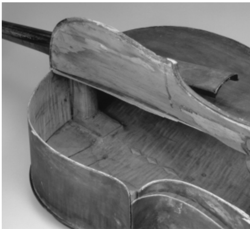
Figure 4. Detail of neck joint and grooved belly from bass viol, Abraham Prescott, Concord, New Hampshire, about 1830–1840. Museum of Fine Arts, Boston, Frank B. Bemis Fund, 1987.19.
