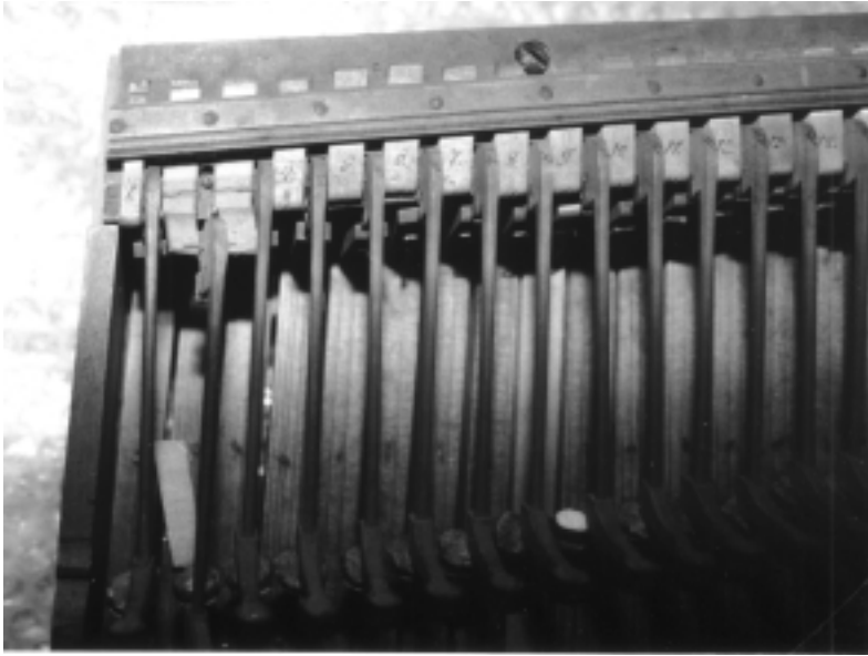
Figure 35. Hammer mounting with leather strips and wedges of an unsigned square piano attributed to Ignatz Kober. Technisches Museum Wien, no. 350. Photo: Sabine Klaus.
