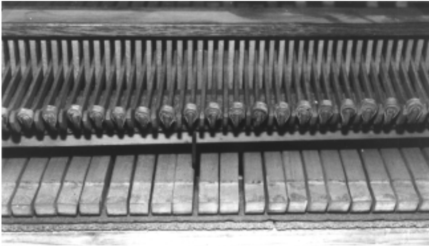
Figure 44. Comb-like rack for pivoting the hammers in the square piano by Johann Friedrich Hoffmann, Cleve. Hammers seen from the back. Smithsonian Institution, National Museum of American History, Washington, D.C., 299,865. Photo: Sabine Klaus.
