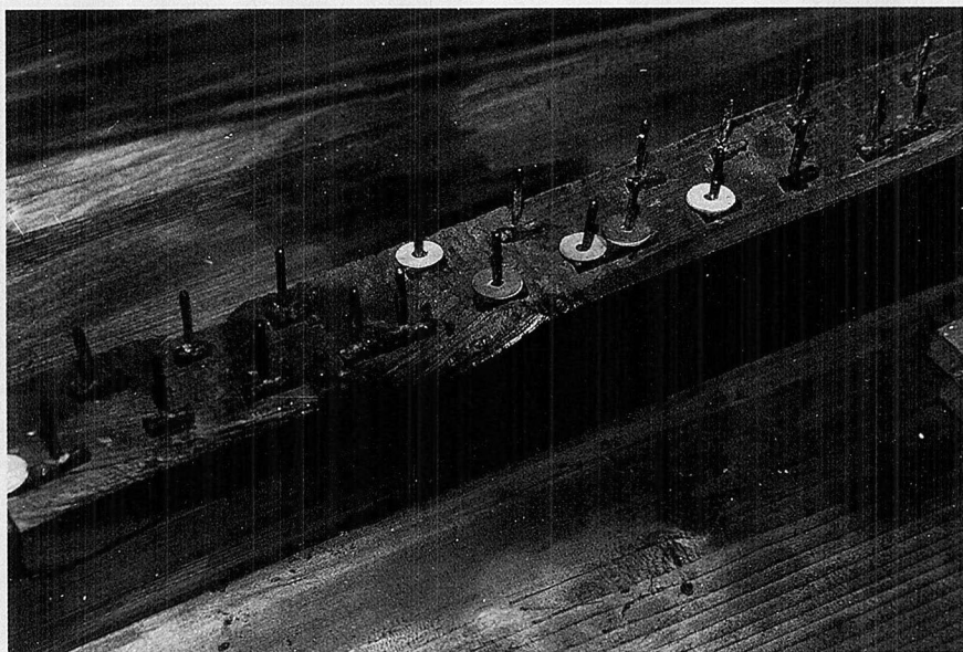
FIGURE 33. Balance rail of the square piano by Gottlob Emanuel Hüfner. Smithsonian Institution, National Museum of American History, Washington, D.C., 332,175. Photo: Sabine Klaus.
