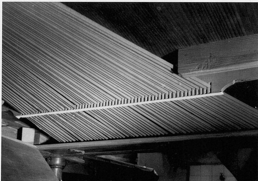
FIGURES 8 and 9. Johann Andreas Stein. Vis-à-vis piano-harpsichord, 1783. The instrument is seen from below, with a panel removed to reveal the system of trackers linking the upper keyboard on the harpsichord end to the piano action at the other end. Photos courtesy Horst Rase.
