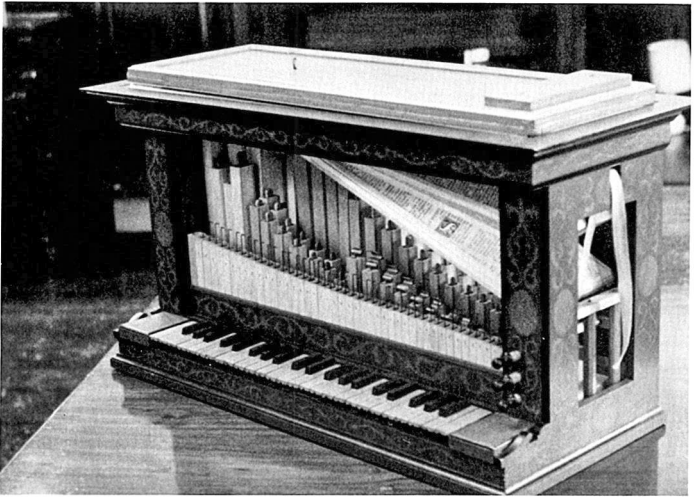
FIGURE 10a. Positive with superior feeder bellows. Reproduction after Haase (1684) by Noel Mander of London, 1978.
