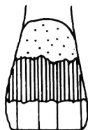
FIGURE 2. Schematic illustration of the second type of scrape found on early bassoon reeds.
