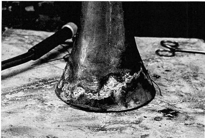
FIGURE 8. The repaired bell of the Bauer trombone (garland and bell rim removed).
